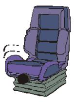
amplify. If the dominant frequencies of the vehicle vibration fall within this amplification range, the seat suspension will make the driver's vibration exposure worse. ISO EN 7096:2000, ISO EN 5007 and EN 13490:2001 provide performance criteria for earth moving machinery, agricultural wheeled tractors and industrial trucks respectively that are designed to ensure appropriate performance of seat suspension.
