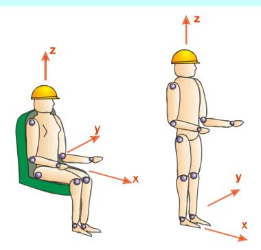
Figure B.2 Vibration measurement axes
