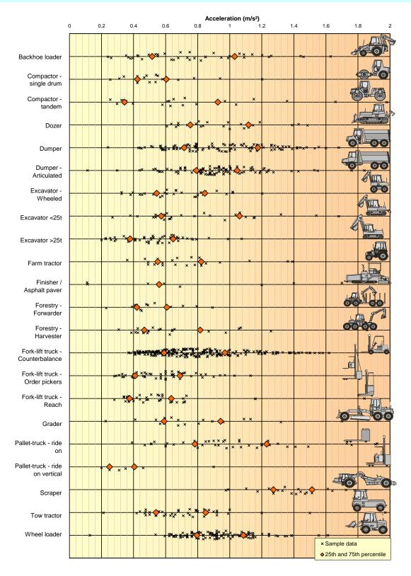
**Figure B.3 Examples of vibration magnitudes for common machines** Sample data based on workplace vibration measurements of highest axis vibration values by INRS INRS (with the assistance of CRAM and Prevencem), HSL and RMS Vibration Test Laboratory between 1997 and 2005. These data are for illustration only and may not be
