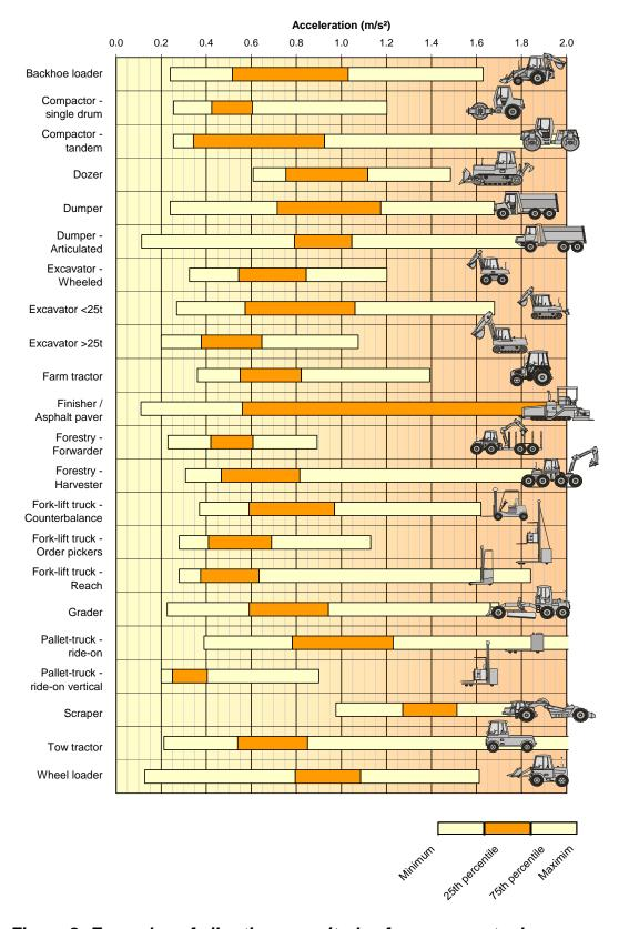
Figure 2 Examples of vibration magnitudes for common tools Ranges of vibration values for common equipment on the EU market. These data are for illustration only. For more details see <u>Annex B</u>.
