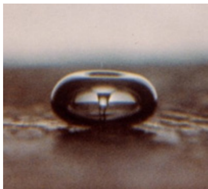
Figure 1. A bubble collapses under an oscillating pressure field. Instead of remaining as a sphere as it collapses, the presence of a solid (brown) wall at the base hinders flow there, so the liquid at the upper wall of the bubble moves faster, accelerating to form a high speed microjet. Image courtesy Prof. L A Crum.
