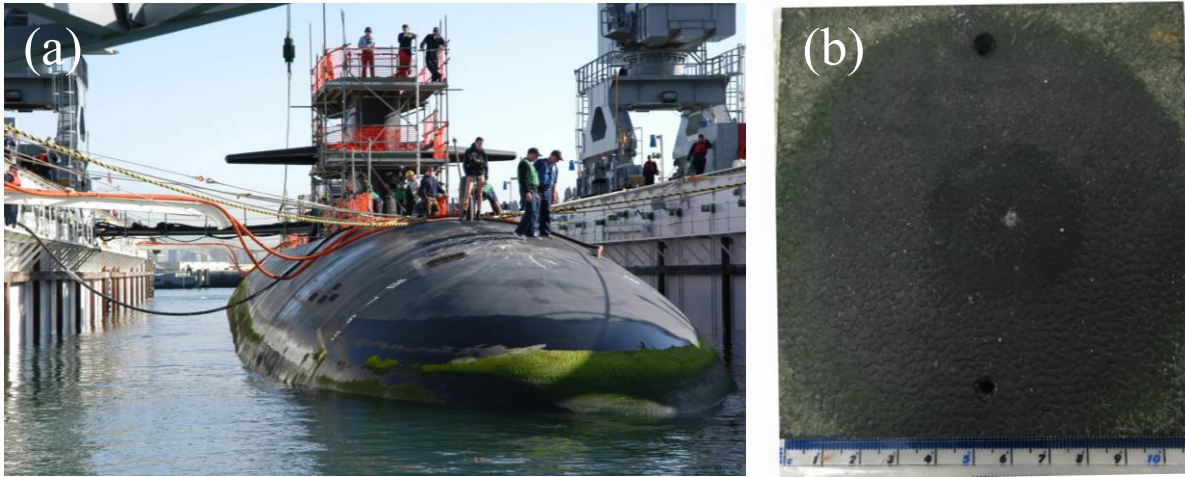
Figure 3. (a) A fast attack submarine, showing significant biofouling that will reduce its speed and efficiency. At the Naval Base Point Loma, Calif. (Jan 10, 2006), the crew of the Navy's only commissioned floating dry-dock, ARCO (ARDM-5), uses mooring lines to pull in Los Angeles-class, fast-attack nuclear submarine, USS Helena (SSN-725). After mooring, the floating dry-dock will blow water out of its ballasts allowing for complete access to the submarine. The crews of ARCO and Helena along with civilian contractors will perform scheduled maintenance procedures on the boat. U.S. Navy photo by Journalist Seaman Joseph Caballero). (b) Damage to a rubber tile caused by removing biofouling from it with a circular rotating brush. The image is not meant to imply that such a cleaner or damage occurs in the situation shown in (a).
