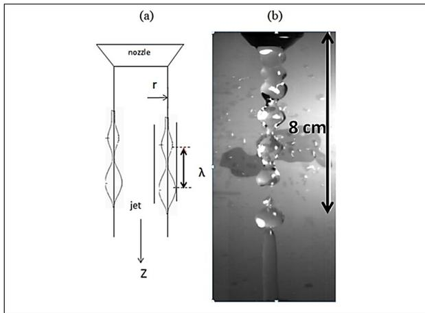
Figure 1. The coordinate system used in the present paper with the axes and a snapshot of the breakup process on a 15 mm diameter of the water stream (measured as the inner diameter at the nozzle) under the action of 134.9 kHz ultrasound.
