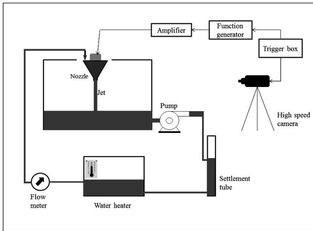
Figure 2. Experimental setup used for observing the surface oscillations formed on the surface of stream with ultrasound propagating through it.
