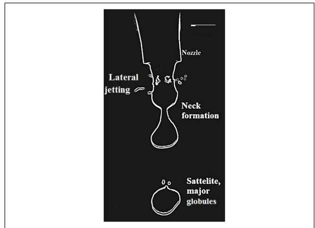
Figure 3. An edge detection technique used to observe the breakup of a water stream exiting a 10 mm inner diameter nozzle activated by 134.9 kHz continuous ultrasound signal.
