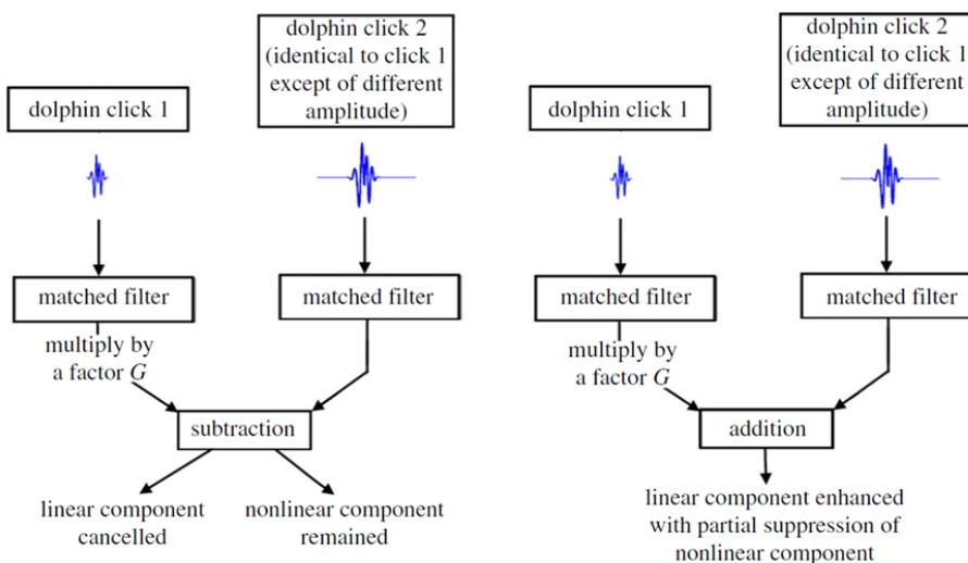
*Fig. 1: Processing scheme by which the echoes from a pair of dolphin-like pulses of different amplitude are processed to enhance/cancel the nonlinear/linear components of the scattering through weighted subtraction and addition of the scattering. The magnitude of the second pulse is greater than that of the first pulse by a factor of  $G$ . From Leighton et al. [5].*
