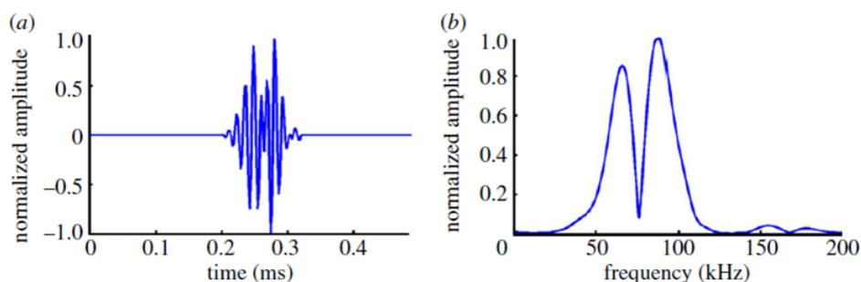
Fig. 2: The pulse used presented in (a) time domain and (b) frequency domain with a peak-to-peak amplitude of approximately 220 dB re 1  $\mu\text{Pa m}$ . From Leighton *et al.* [5].
