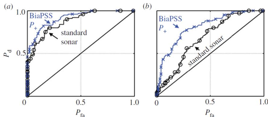
Fig. 4: ROC curves computed from (a) the tank data and (b) simulated data, for the scenario described in this paper. The results for BiaPSS  $P_+$  (cross symbols) are compared with the results for standard sonar processing (circles). The solid line without symbols shows the  $45^\circ$  line, which represents the most useless form of sonar (see text). From Leighton et al. [5].
