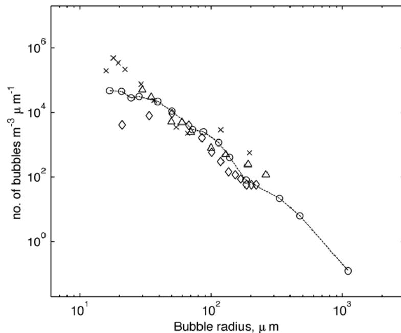
Figure 2. Plot of the acoustically measured bubble size distribution (black circles with dashed line). This population estimate represents the spatially averaged bubble density between two hydrophones, at mean depths of 0.8 m and 2.54 m. Historical measurements are also shown. The diamonds are those of Johnson and Cooke [11], the triangles are those of Breitz and Medwin [12] and the crosses are those of Phelps and Leighton [13].
