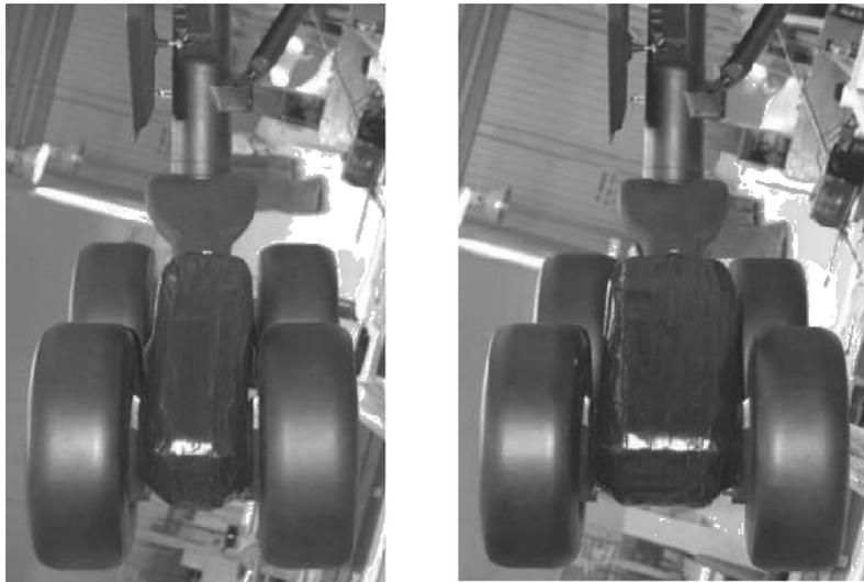
**Figure 5:** Bogie fairings in combination with torque link fairings for different wheel spacing.
