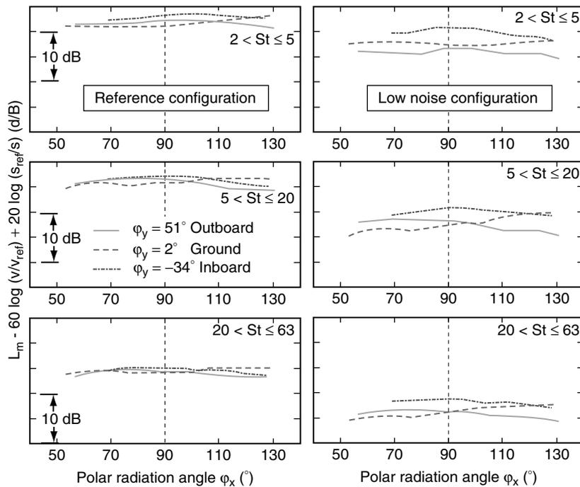
**Figure 12:** Polar directivities of non-dimensional 1/3-oct. band noise levels in different bands of Strouhal number for the reference, the TIMPAN low noise configurations and different azimuthal (sideline) radiation angles  $\phi_y$ , respectively.
