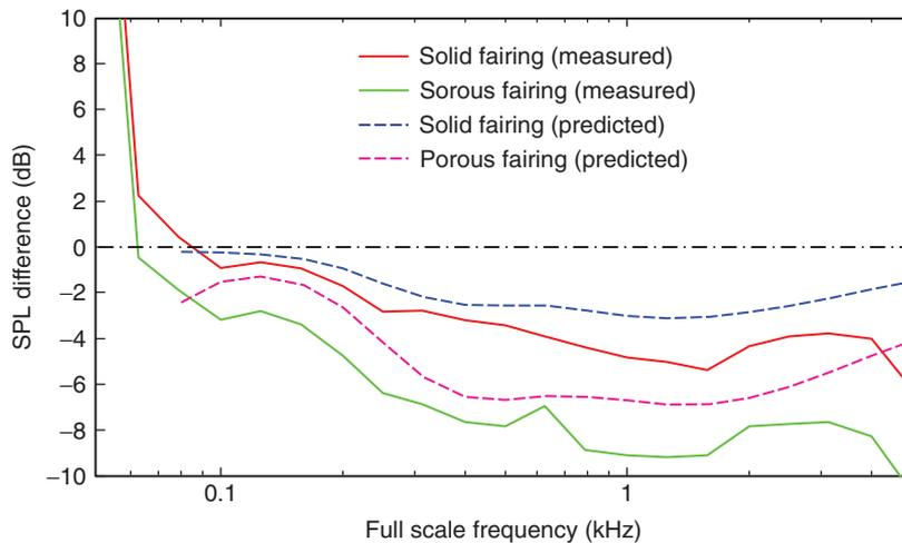
**Figure 15:** Predicted and measured effect of installing either a solid or porous bogie fairing and ramp fairing on the standard gear with the TIMPAN folding side-stay.
