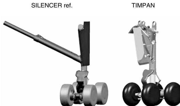
**Figure 1:** Comparison of SILENCER and TIMPAN main landing gear concepts.
