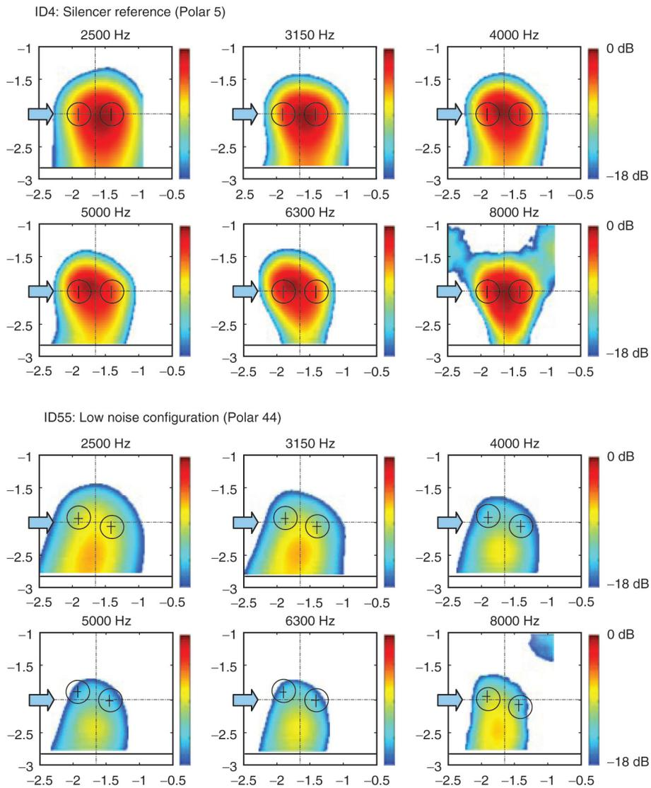
**Figure 11:** Comparison of noise source distributions from a “side view” for the reference configuration and the TIMPAN low noise configuration and different 1/3-oct. band frequencies, respectively (wind speed from left to right; same level scales for the two configurations at identical frequency but autoscaling for different frequencies).
