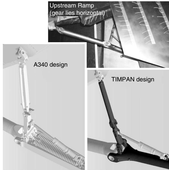
**Figure 2:** TIMPAN side-stay design and upstream ramp.
