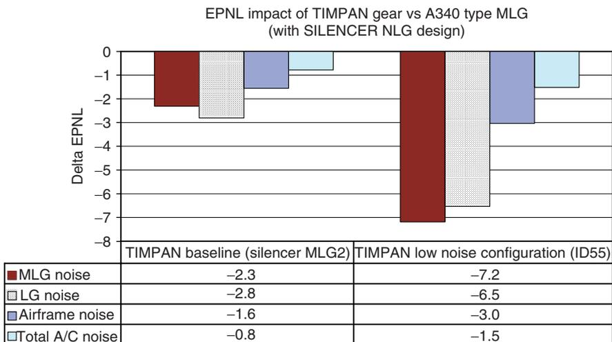
**Figure 17:** Impact on EPNL for approach conditions of the TIMPAN low noise main landing gear design vs the SILENCER (reference) gear design and the original A330/A340 gears, respectively.
