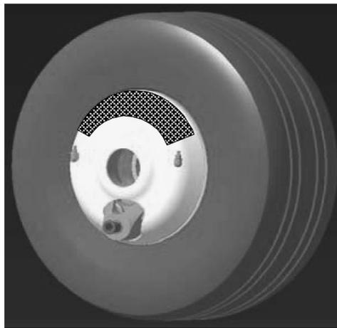
**Figure 3:** Brake faring with mesh type insert for brake cooling.
