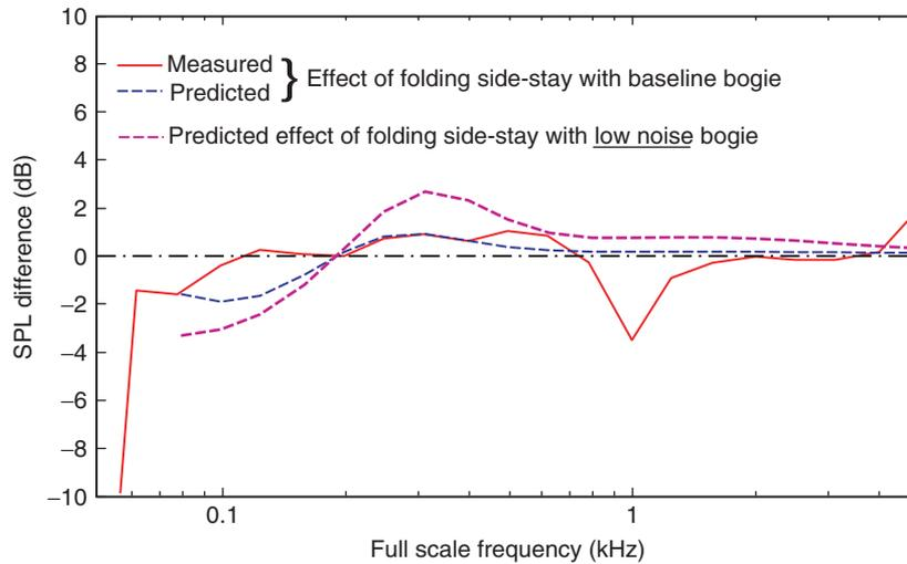
**Figure 16:** Noise increase due to changing from the SILENCER telescopic side-stay to the TIMPAN folding side-stay with the bogie in its reference configuration or its low noise configuration, respectively.
