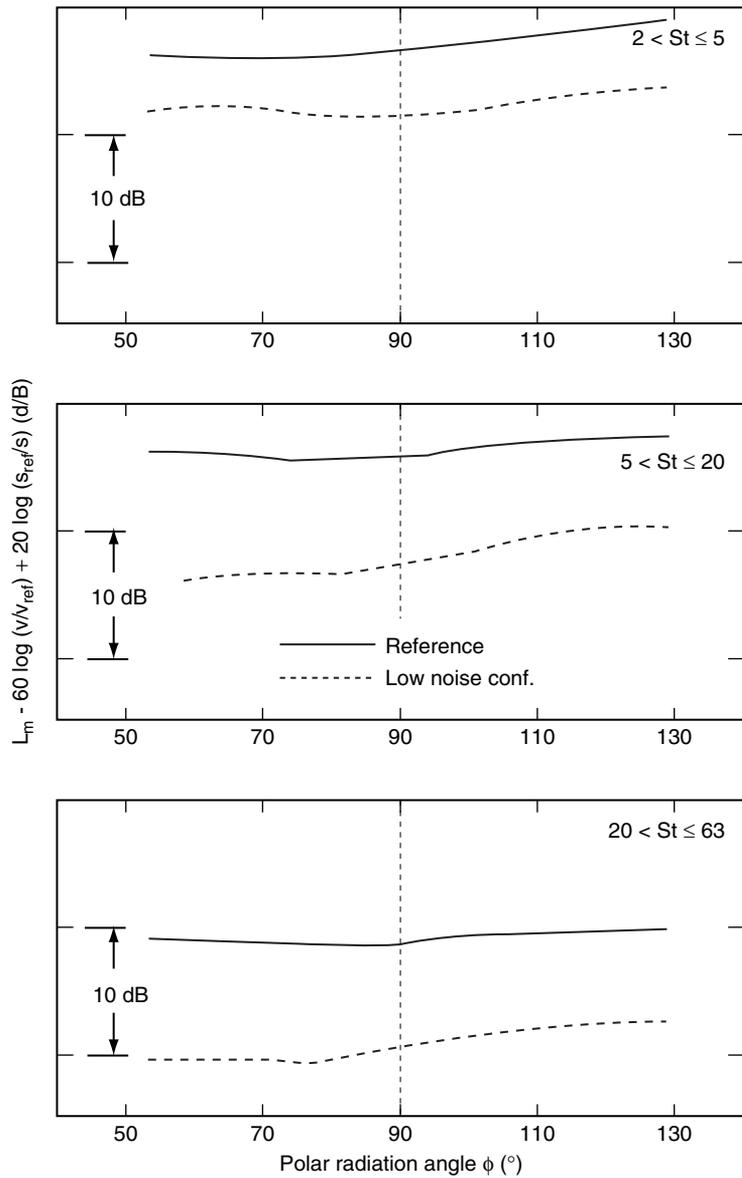
**Figure 10:** Comparison of polar directivities of normalized 1/3-oct. band noise levels in different bands of Strouhal number for the reference and the TIMPAN low noise configuration.
