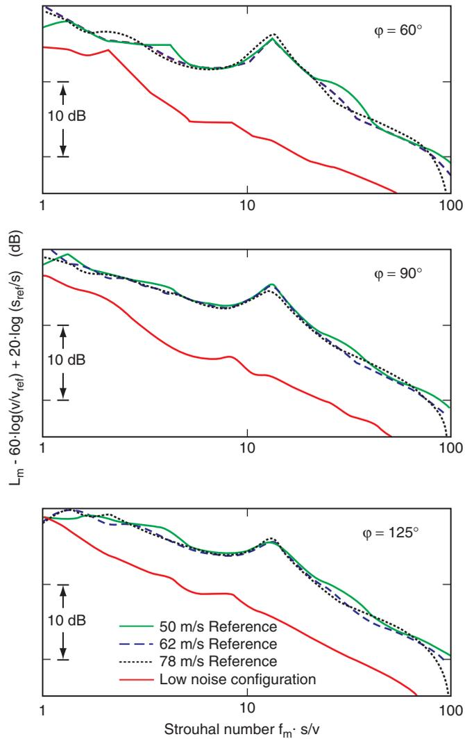
**Figure 9:** Comparison of normalized 1/3-oct. band noise spectra for the reference and the TIMPAN low noise configuration at different polar radiation angles.
