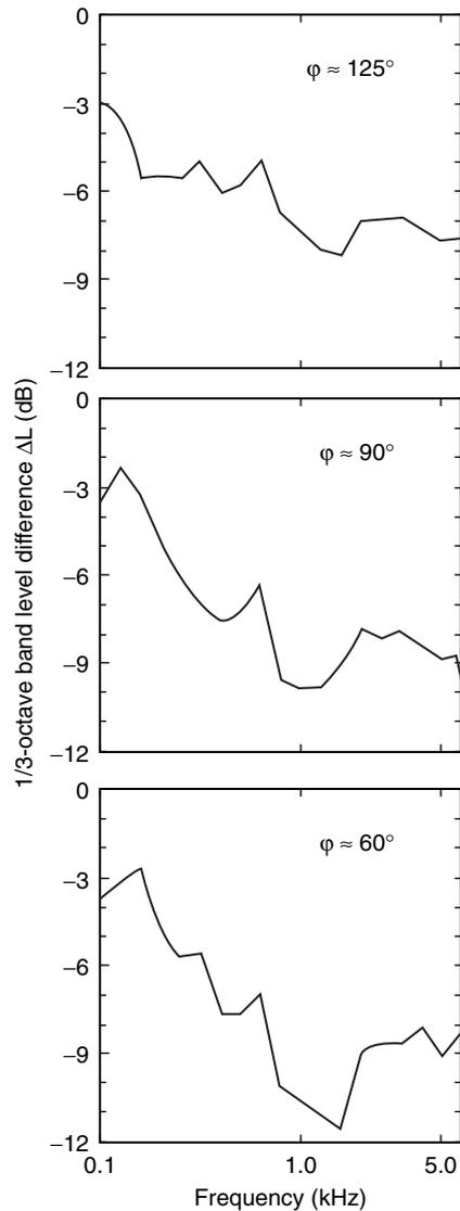
**Figure 14:** Noise reduction potential vs full scale frequency of the TIMPAN low noise configuration in comparison with the reference configuration.
