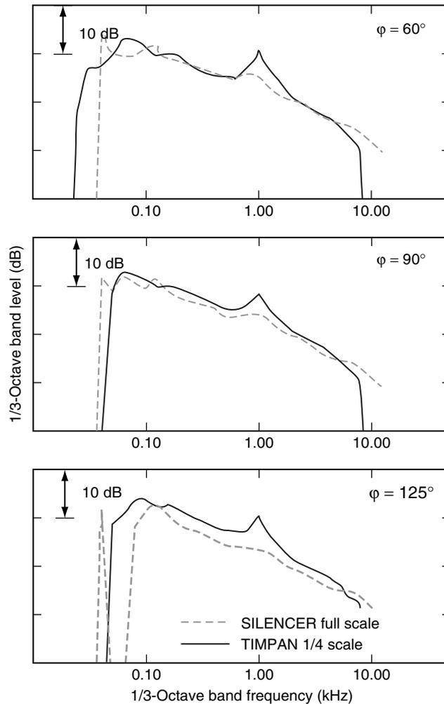
**Figure 8:** Comparison of normalized 1/3-oct. band level spectra for the TIMPAN  $1/4$  scaled model gear in its reference configuration with the spectrum for the original full scale SILENCER advanced gear at different polar radiation angles.
