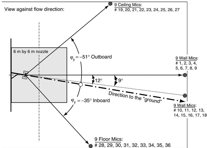
**Figure 7:** Selected farfield microphone positions on the wind tunnel side wall, the ceiling and the tunnel floor.
