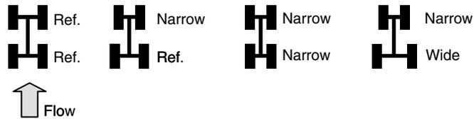
**Figure 4:** Schematic of selected combinations of forward and rear wheels' spacing.
