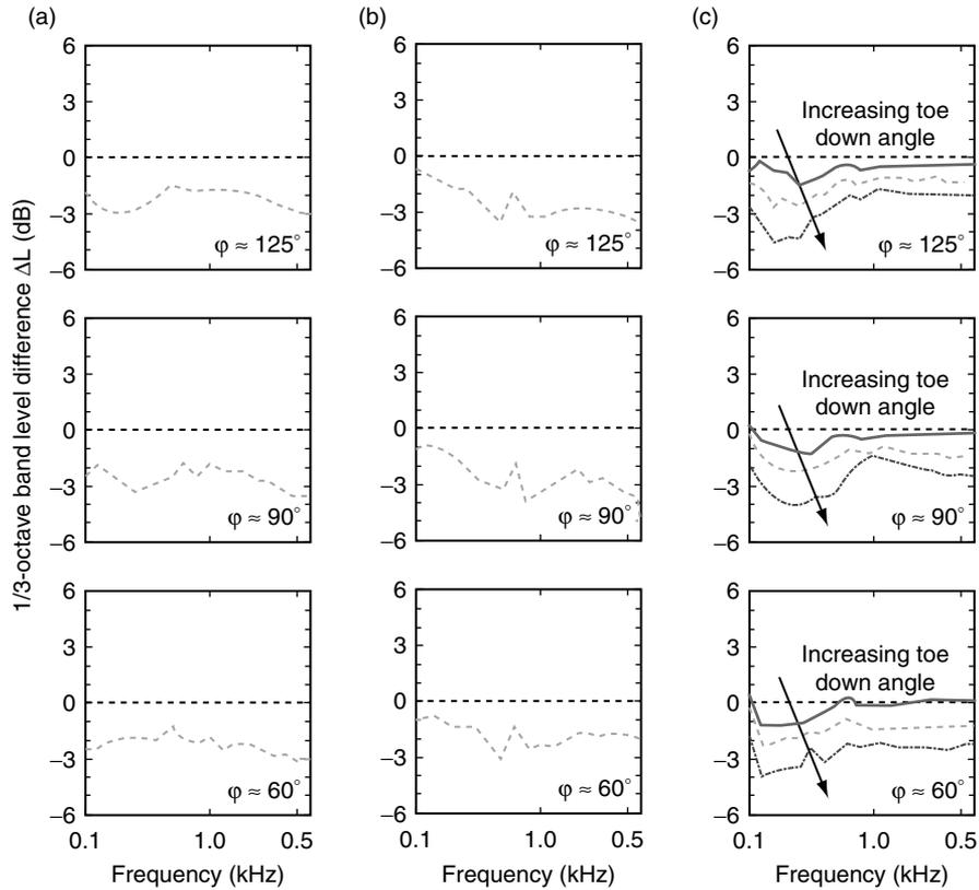
**Figure 13:** Effects of (a) porous bogie fairing and (b) porous torque link fairing w.r.t. solid fairings and (c) of bogie inclination angle.
