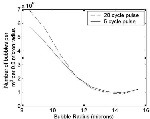
Figure 3. Estimated bubble populations for 5 and 20 cycles pulse. The measurement was made in a wind speed of 14-15 mph off shore breeze, with a water temperature of 11 °C and at a depth of ~1 m. The pH of the water was 6.12 and the dissolved oxygen content was 5.3 mg/litre. Estimation of bubble population was made by inversion of attenuation measurements following the method described in [4-6].
