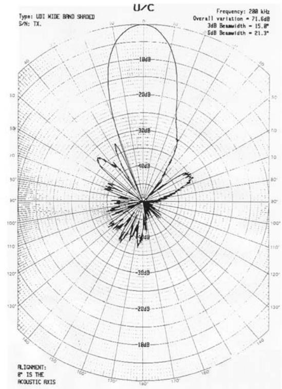
Figure 4. Beam Pattern at 200 kHz for source used in Hurst Spit sea trial: 3 dB beamwidth=15.8°; 6 dB beamwidth=21.3°.
