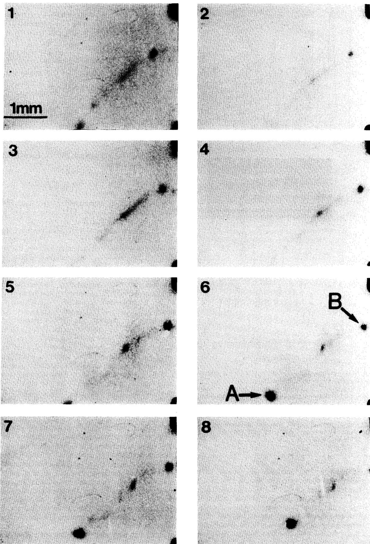
**Figure 7** Eight frames selected from a film shot at  $2000 \text{ frames s}^{-1}$  showing a microstreamer of tiny bubbles propelled between two larger bubbles by radiation forces. The source is the bubble labelled A. Bubble fragments are sheared off from the surface of A; they travel in the microstreamer under the influence of the mutual Bjerknes force, to coalesce with the bubble marked B. Acoustic parameters as for *Figure 5*
