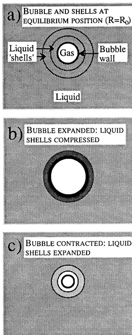
**Figure 4** The 'shell' effect: the bubble and two of the liquid shells surrounding it are shown. (a) The bubble is at equilibrium size; (b) the bubble expands, and the liquid shells contract; (c) the bubble contracts, and the liquid shells dilate
