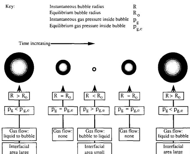
**Figure 3** The 'area' effect. One oscillatory cycle of the bubble pulsation is illustrated. The pressure within a pulsating bubble and the surface area of the transfer (the bubble wall) both oscillate about an equilibrium value, causing a mass flux imbalance
