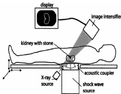
**Figure 1.** Schematic of Lithotripsy.
