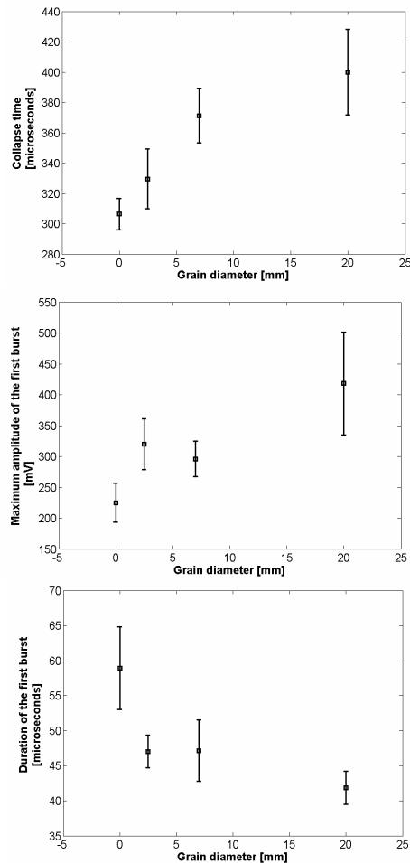
**Figure 7.** (a) Collapse time  $t_c$  (b) Maximum amplitude of the first burst. (c) Duration of the first burst. The errorbars equal the ratio between the maximum error and the root square of the number of measurements per stone sample. A grain diameter of zero indicates that the table-tennis ball was filled with tap water only.
