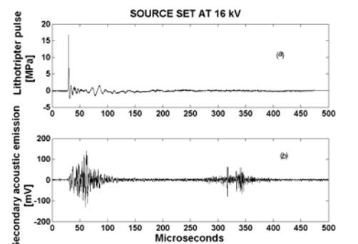
**Figure 4.** (a) Experimental lithotripter pulse at 16 kV. (b) Secondary acoustic emission detected using the NPL cavitation sensor.
