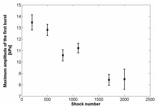
**Figure 8.** Trend of the maximum amplitude of the first burst during a clinical treatment. The errorbars equal the ratio between the maximum error and the root square of the number of measurements per shock.
