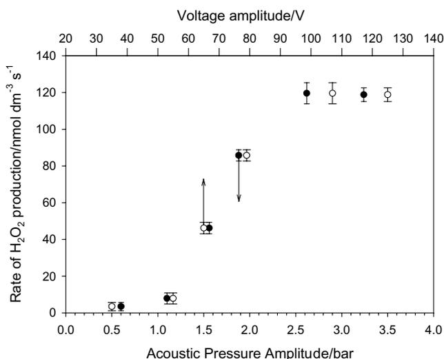
Fig. 5. Plot showing the rate of hydrogen peroxide production as a function of the acoustic pressure amplitude<sup>1</sup> (●) or drive voltage amplitude (○) at 124 kHz. Error bars represent one standard deviation calculated using repeat measurements.
