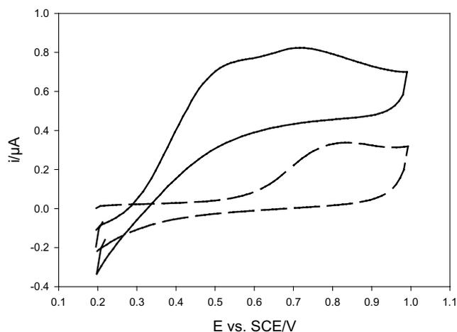
Fig. 1. Plot showing the cyclic voltammograms of a 0.5 mm diameter Pt electrode in pH 5.5 citrate/phosphate buffer. (---) represents the voltammetry of the buffer alone while (—) represents the voltammetry of the buffer with 1 mmol dm<sup>-3</sup> H<sub>2</sub>O<sub>2</sub> added. The voltammetry was recorded under aerobic conditions at 50 mV s<sup>-1</sup> and at 25 °C.
