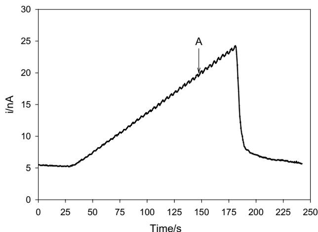
Fig. 4. Plot showing the current recorded as a function of time for the electrochemical detection of sonochemically generated hydrogen peroxide. The ultrasound was turned on at time  $t = 0$  s. The potential of the electrode was held at  $+0.8$  V vs. SCE. The ultrasonic frequency was 125 kHz and the voltage amplitude was 110 V corresponding to acoustic pressure amplitude of 2.45 bar.<sup>1</sup> An excess of catalase was added at 'A'.
