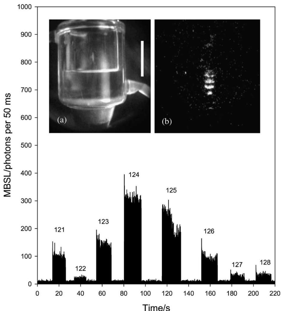
Fig. 3. Plot showing the MBSL output of the cell as a function of time as the ultrasound irradiation of the cell was chopped on and off. The irradiation frequency is reported in the figure (in kHz). The insert in the figure shows images recorded of the sonochemical reactor. Image (a) corresponds to the cell pictured in the light while image (b) shows the MBSL activity at 123 kHz recorded under dark room conditions. The scale bar represents 4 cm.
