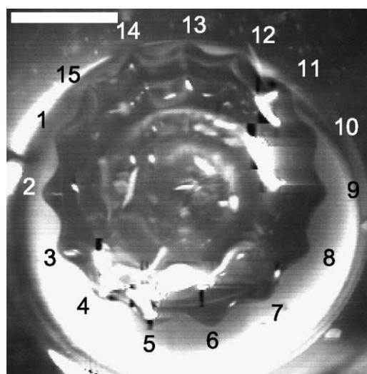
Fig. 1. Image recorded of a tethered gas bubble driven into oscillation by an acoustic driving field. Surface waves are clearly seen on the gas/liquid interface. The bubble was driven at 1.297 kHz. The scale bar represents 2 mm. The image is annotated to indicate the mode excited ( $n = 15$ ).
