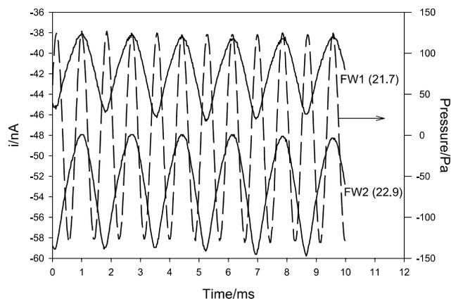
Fig. 5. Plot showing the current (—) for the Faraday wave electrochemical signals labelled 'FW' on Fig. 4b. (---) represents the acoustic pressure measured simultaneously in the presence of the bubble for reference. The acoustic pressure amplitudes are given in parenthesis while the drive frequency was maintained at 1.167 kHz. All other experimental conditions are described in Fig. 2.
