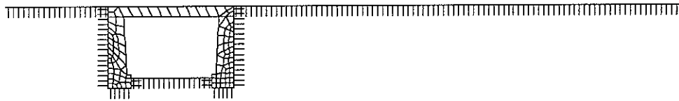
Figure 16. Mesh for the cut-and-cover tunnel model showing boundary element normals.
