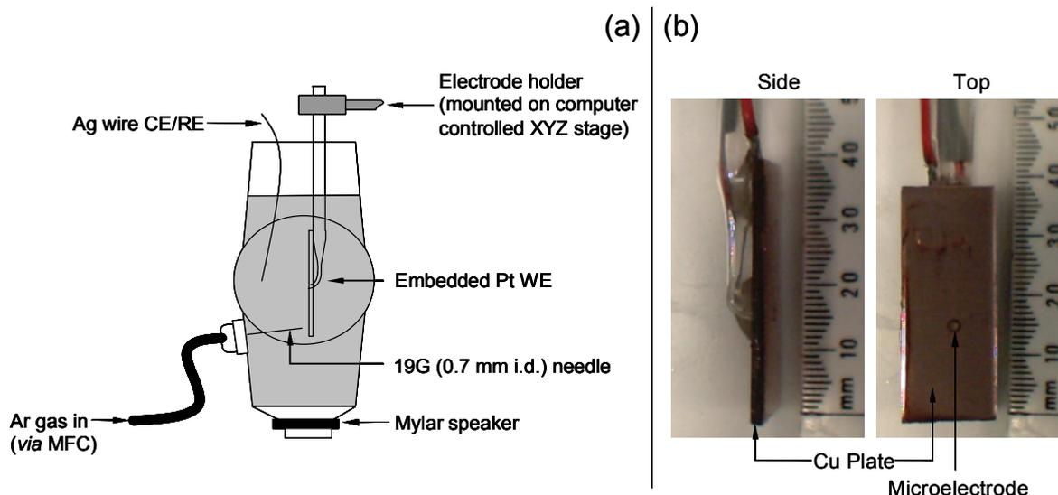
Figure 1a. Experimental setup. b. Side and top views of the embedded 50 µm diameter Pt microelectrode.
