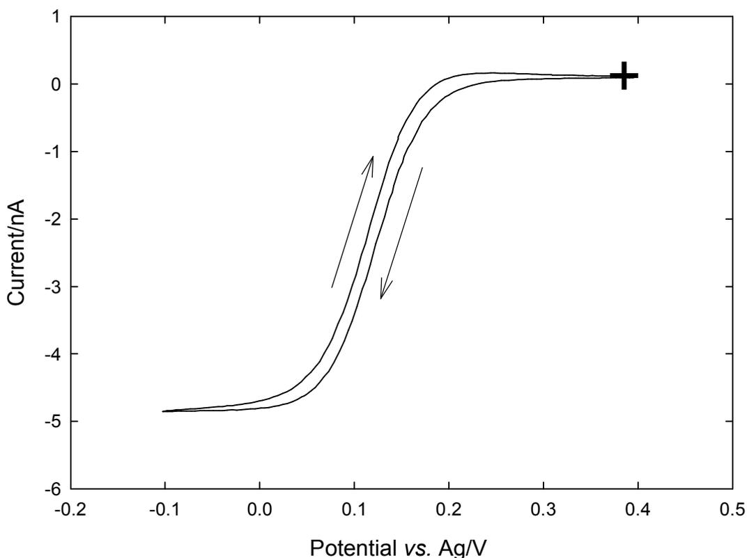
Figure 2. Cyclic voltammogram recorded at a 25  $\mu\text{m}$  diameter Pt microelectrode in a solution of 5 mM  $\text{K}_3\text{Fe}(\text{CN})_6$  and 0.1 M  $\text{Sr}(\text{NO}_3)_2$  to which 50 % (by weight) sucrose was added. The plus symbol (+) indicates the start position and the arrows indicate the direction of the scans. The scan rate was 5  $\text{mV s}^{-1}$ . The experiment was carried out at 25  $^\circ\text{C}$  and under aerobic conditions.
