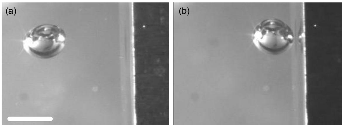
Figure 4. Photographs of rising bubbles in the absence (a) and presence (b) of insonification at 2.86 kHz. The pressure amplitude measured in the centre of the cell in the absence of the electrode and bubble injection was 322 Pa. In both cases all other conditions are identical. The dark area at the right of each frame is a copper plate. The scale bar in (a) represents 2 mm.
