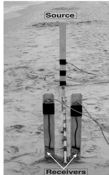
Fig. 6. SPADE probe deployment during fieldwork, with receivers positioned at approximately the same S-R separation, lying on either side of the central line, which is marked by the measuring pole.
