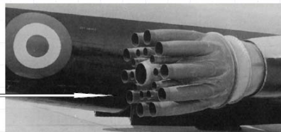
21-tube nozzle for a 1960's Boeing 707
