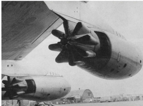
8 corrugated silencers for Conway engines on a 707-420
