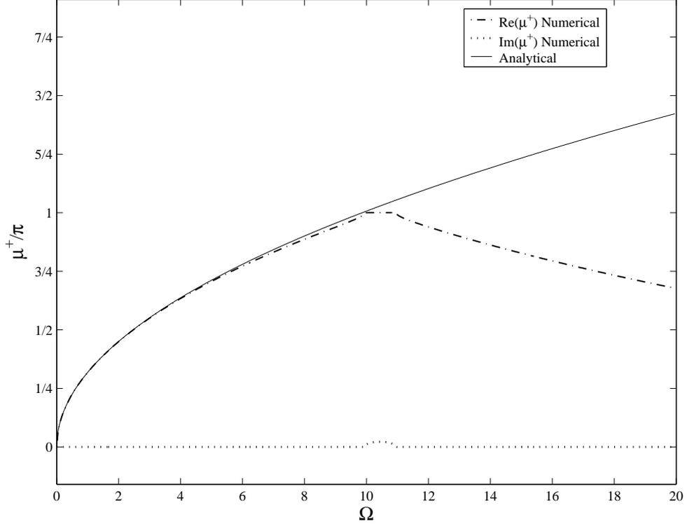
Figure 7: Isotropic plate. Complex-valued dispersion curve for  $\theta = 0$ .
