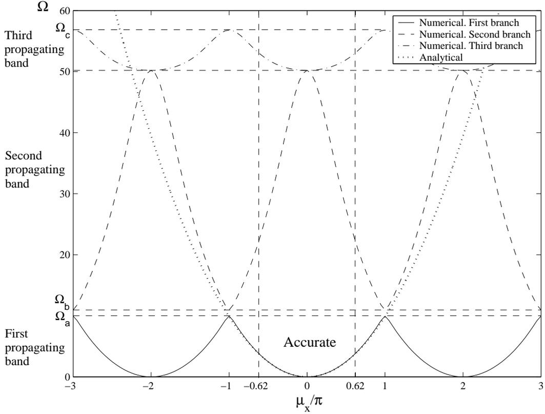
Figure 4: Real-valued dispersion curves for  $\theta = 0$ . Numerical and analytical curves.
