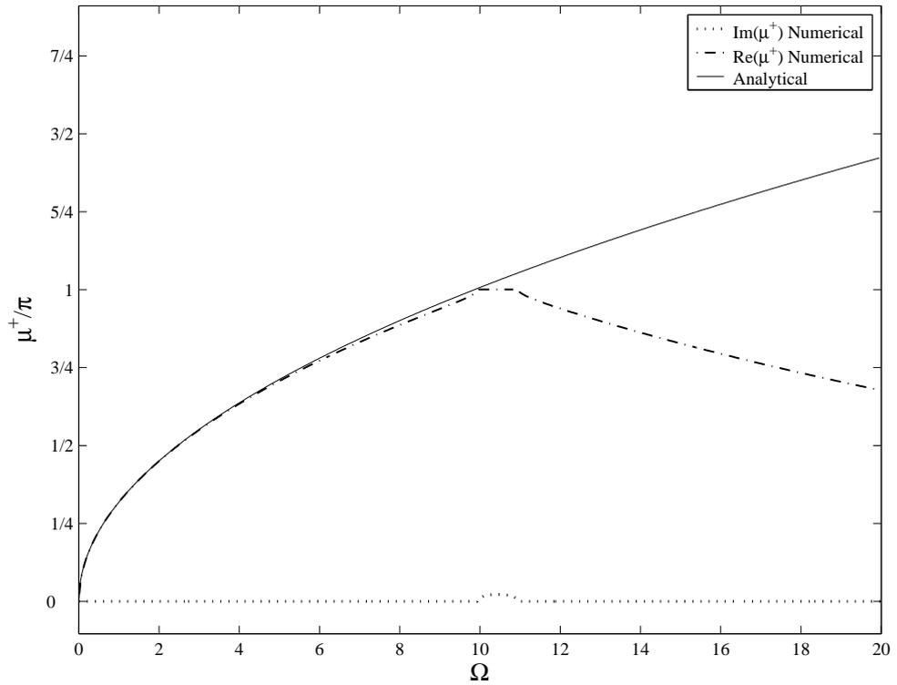
Figure 16: Orthotropic plate. Complex-valued dispersion curve for  $\theta = 0$ .
