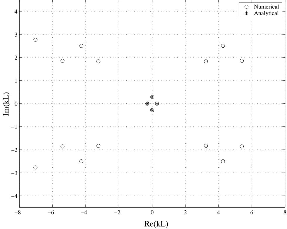
Figure 9: Isotropic plate. Location of the nondimensional wavenumber –obtained solving equation (15)– in the complex  $(\text{Re}(kL), \text{Im}(kL))$  plane.  $\theta = \arctan(1/2)$ ,  $\Omega = 0.0837$ .
