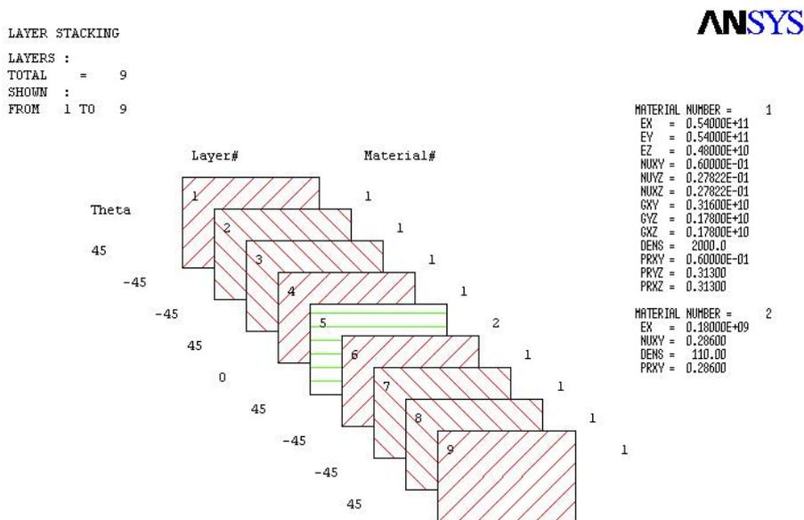
Figure 29: Sandwich shell: layers stacking and material properties.
