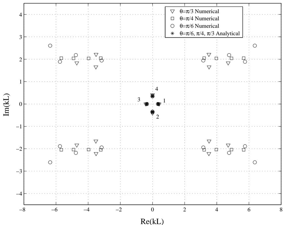
Figure 17: Orthotropic plate. Location of the nondimensional wavenumber in the complex ( $Re(kL)$ ,  $Im(kL)$ ) plane,  $\Omega = 0.1003$ .
