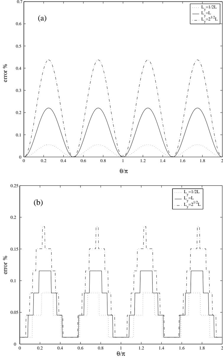
Figure 8: Isotropic plate. Relative error in the estimated frequency, figure (a), and in the wavenumber, figure (b), as a function of the wave propagation direction  $\theta$ ,  $kL = 0.2893$ ,  $\Omega = 0.0837$ .
