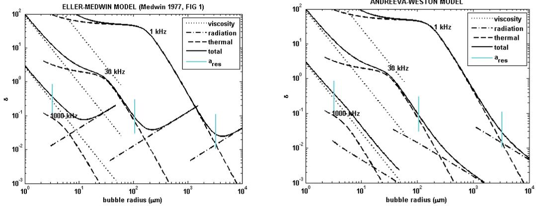
Fig.1: Theoretical damping parameter  $\delta$  versus bubble radius for acoustic frequencies 1 kHz, 30 kHz and 1 MHz; the resonant bubble radius is marked for each frequency using a vertical grey (cyan) line; The contribution due to acoustic radiation is shown as a dash-dotted line (-.-). left: Wildt-Devin-Eller-Medwin; right: Andreeva-Weston.
