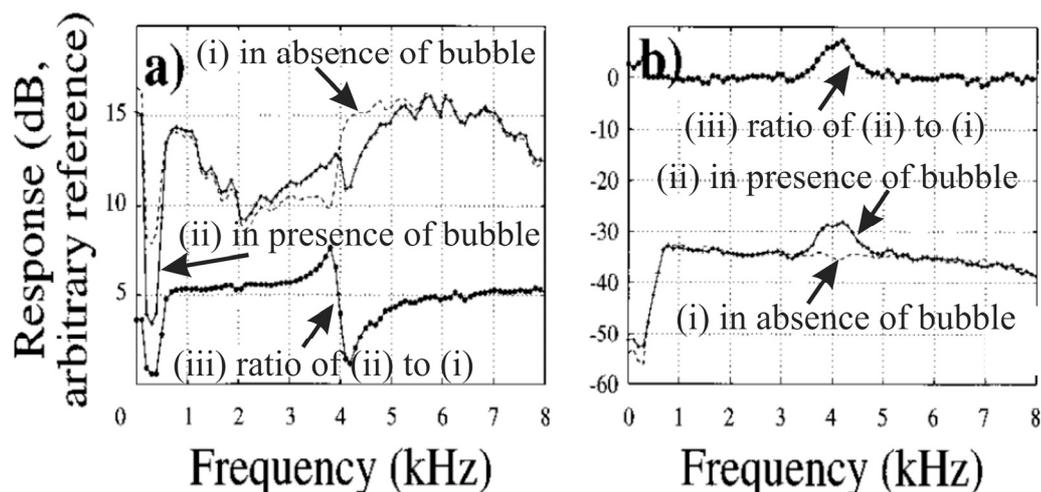
Fig.3: Plots with 98 Hz resolution of (a) the modulus of voltage transfer function and (b) coherence, calculated from the (a) signal from the B&K8103 hydrophone and (b) the heterodyned signal from the Panametric V302 receiver shown in Fig. 2. A rising stream of bubbles of radius 800  $\mu\text{m}$  was subjected to broadband insonification by a band limited 1–8 kHz pseudo-random noise sequence.
