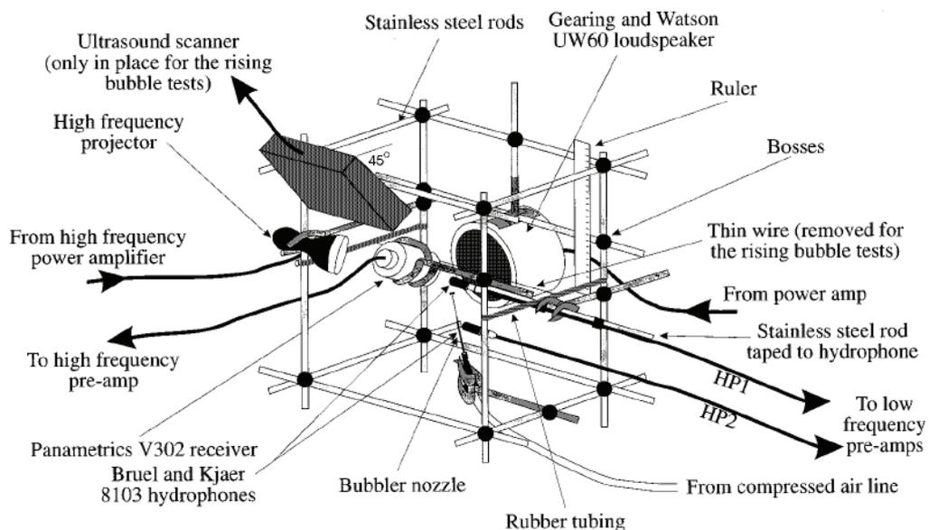
Fig.2: Apparatus used by Leighton et al. [11] for characterisation of the resonance.
