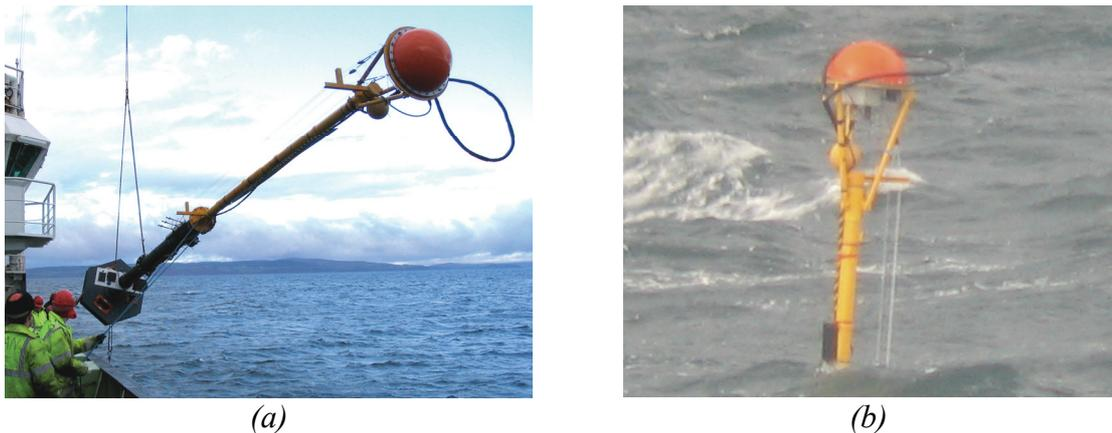
Fig. 6: (a) The 11 metre spar buoy being deployed off RRS Discovery. (b) The spar buoy as it sits in the sea.
