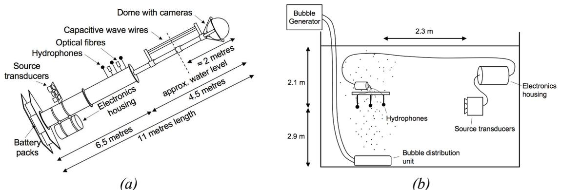
Fig. 1: (a) Schematic (not to scale) of the buoy which, at sea, is vertical with the dome at the top. (b) Tests in the  $8 \times 8 \times 5 \text{ m}^3$  AB Wood tank (Hydrophone spacing: 0.31 m).
