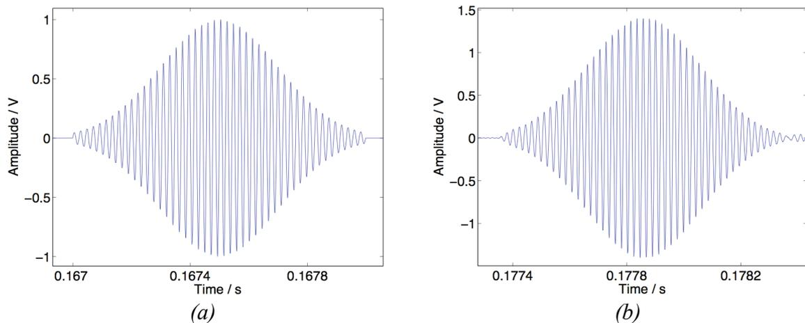
Fig. 3: (a) The outgoing 46 kHz pulse signal that was transmitted to the power amplifiers prior to output into the water. (b) The same pulse as measured by the hydrophones in bubble-free conditions.
