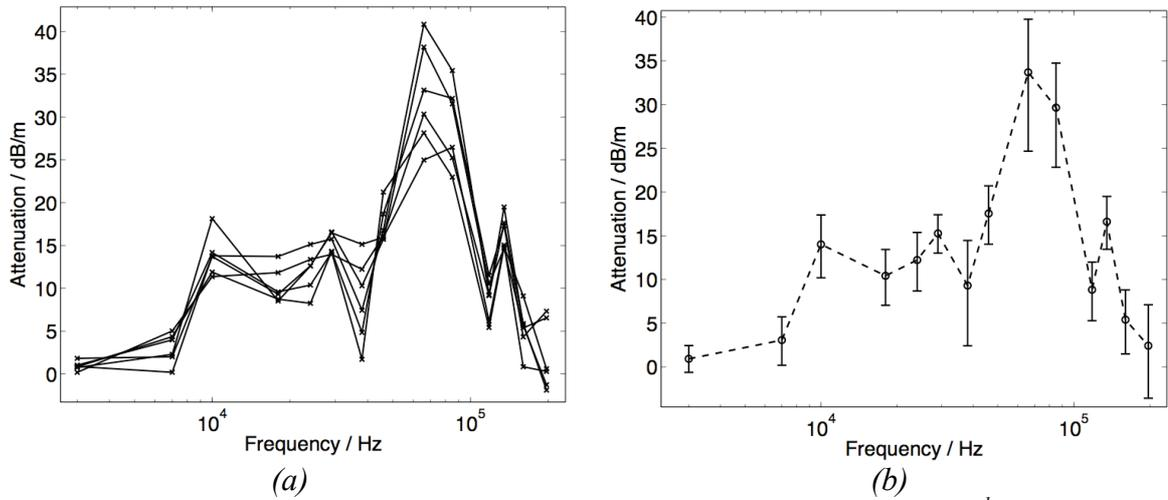
Fig. 4: (a) The additional attenuation due to bubbles between the 1<sup>st</sup> and 3<sup>rd</sup> hydrophones, which were at a distance of 0.62 metres apart. The figure shows 6 separate readings, spaced approximately 1 second apart. (b) The mean of the 6 values shown in (a) (calculated from linear pressure data, not dBs). The error bars represent 1 standard deviation from the mean of the 6 values and also take into account the uncertainty of the hydrophone calibrations.
