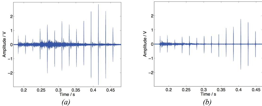
Fig. 2: (a) The pulse train measured at the second hydrophone with no bubbles present. (b) The increased attenuation at the same hydrophone when there are bubbles present.
