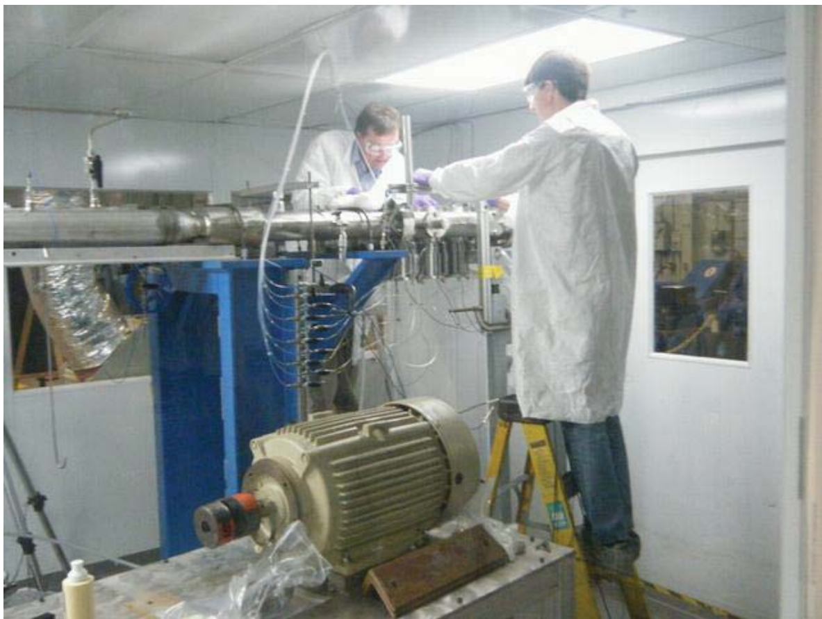
Figure 11. The author and a member of ORNL staff (Mark Wendel) fitting the bubble detectors to the mercury-filled steel pipelines of SNS TTF.
