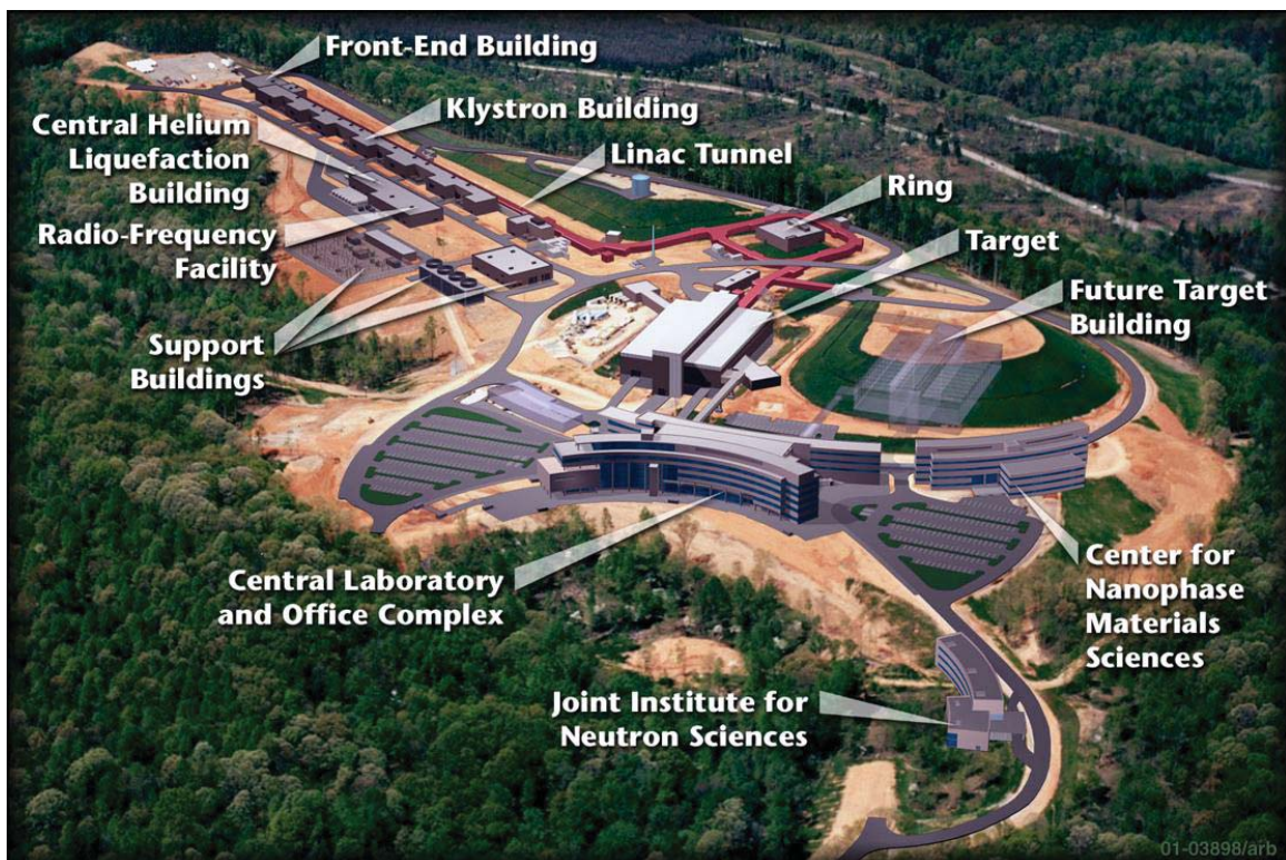
Figure 10. Schematic of the Spallation Neutron Source at Oak Ridge National Laboratory, Tennessee. The hydrogen ions for the linear accelerator are generated in the 'front end' building at the top left of the picture, and are accelerated down the linear accelerator (shown in red) to the ring, where protons are accumulated. During repeated circulation of the ring, more protons are added to 'paint out' the complete 200 mm x 70 mm elliptic proton beam. When this is complete (which occurs 60 times per second), the proton pulse is released into the 'target' building, the centre of which houses the sarcophagus in which the actual mercury target is housed. A possible future target building is shown in ghost outline (image courtesy of ORNL).
