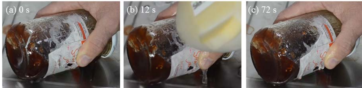
Figure 8. Removal by the UAS of glue used to attach label to jam jar. The video of this is available at: https://www.youtube.com/watch?v=0H3ZE9IrgoQ .
