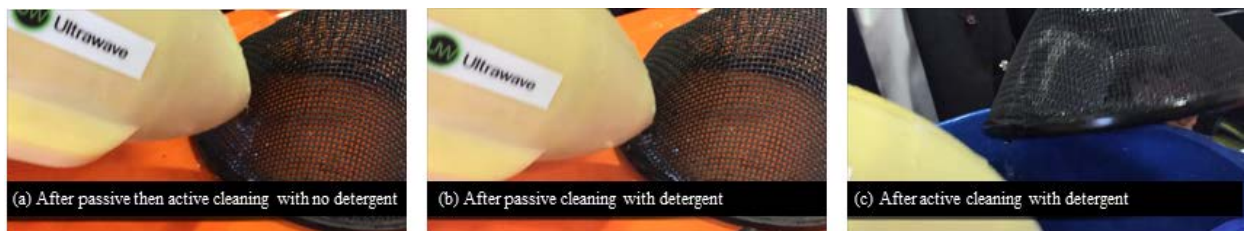
Figure 11. Cleaning part of the wire mesh of an air intake cover after it has been in service on a train. (a) Cold water without ultrasound and without detergent is passed through the StarStream device onto the surface, but produces no visible cleaning. (b) A cold water stream that is free of detergent, and has no ultrasound, is passed onto the surface after household detergent has been sprayed onto the surface. No visible cleaning occurs. (c) A cold water stream that is free of detergent, but has ultrasound in it, is passed onto the surface after household detergent has been sprayed onto the surface. Clear cleaning occurs. The video of this is available at:
