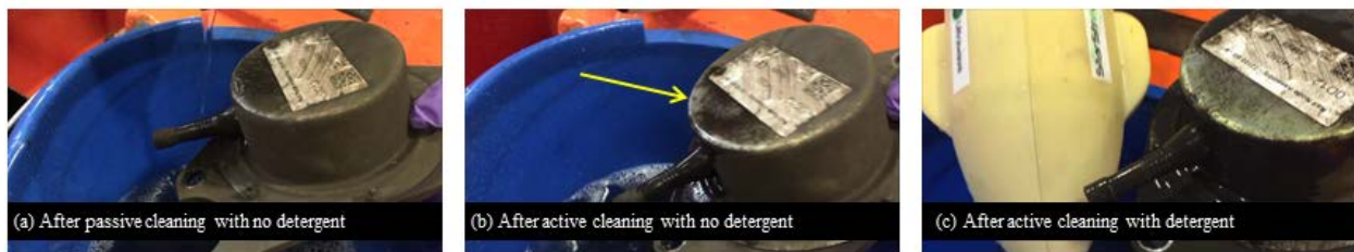
Figure 10. Cleaning part of a sensor (the flat region below the label) after it has been in service on a train. (a) After cold water without ultrasound or detergent is passed through the StarStream device onto the surface. (b) After cold water without detergent but with ultrasound is passed onto the surface: the yellow arrow indicates some cleaning. (c) Some household detergent is sprayed on the surface and then it is treated with the UAS (there is no detergent in the stream that issues from the nozzle): the surface is cleaned. The video of this is available at:
