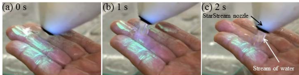
Figure 5. The StarStream device is shown removing contaminant from the author's hand (the timings in the slide are approximate) using cold water without additives. The video of this will be made available via http://www.southampton.ac.uk/engineering/research/projects/starstream.page?
