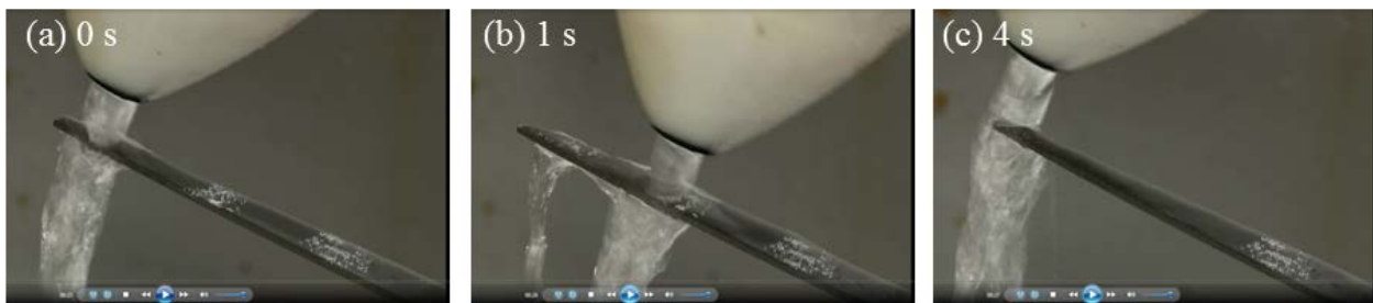
Figure 7. Removal by the UAS of aluminum oxide powder from the grooves in a workshop file. The video of this will be made available via http://www.southampton.ac.uk/engineering/research/projects/starstream.page? .
