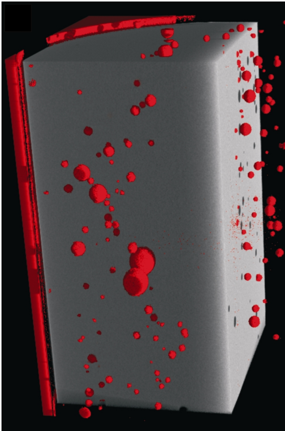
Figure 1. Image generated through CT scanning of a vertical core through bubbly gel (described in reference [49]), used for validation purposes during the construction of the device described in this paper. In the image, the host gel near the edges of the quadrant has been clipped back to show the presence of the bubbles. For scale, the largest bubble visible has a diameter of \sim 1 mm.
