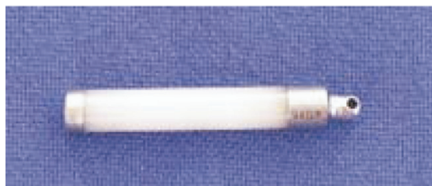
Fig 1. The radiofrequency microstimulator (actual size, 17×2.4mm) showing the eyelet used for attachment on the suture.
