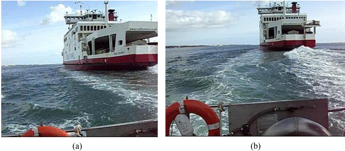
Figure 4. Approaching the wake of the Red Funnel ferry just prior to taking sonar records of Fig. 5. The commercial depth sounder (Wheel house unit: Simrad CR50 with Transducer: Simrad combi C50/200 dual 50 kHz / 200 kHz operating at 200 kHz) fitted to the RV Bill Conway could not function in this wake.
