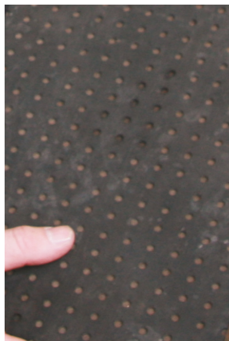
FIG. 8. (Color online) A piece of anechoic tiling from a WWII German U boat. The tiling was designed in response to the effectiveness of the Allied anti-submarine activities, which the Germans attributed to advances in Allied sonar, but which is likely to have been due to other factors (including the cracking of the Enigma Code). The far side of the tile is smooth, but the side visible in the picture was glued to the hull, trapping air in its circular pores. The technique is acoustically effective, though in early versions the tiles debonded from the hull under pressure cycling.
