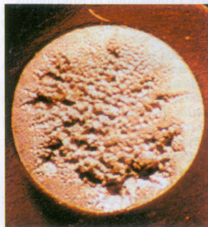
Figure 2. Picture showing the effect of cavitation induced erosion of an aluminium surface. The aluminium substrate is 2mm in diameter, and was highly polished before immersion in a power ultrasound field.
