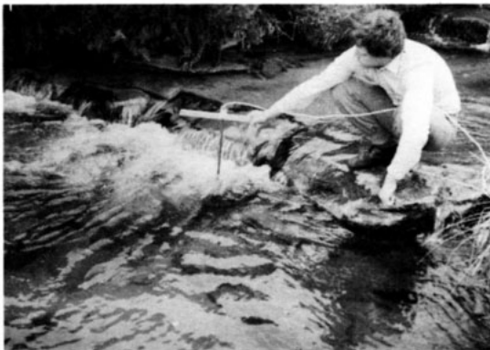
Figure 7 One of the authors (TGL) recording sound emitted from a brook running from Kinder Scout in the Peak District (Derbyshire, UK). The hydrophone is mounted at the end of the paxolin rod. The lead runs to the recorder (not shown) where the sound signals are monitored by the second author.
