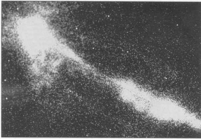
Fig 1 A photograph, taken through the image intensifier, of sonoluminescence in a 90% glycerine/10% water mixture, occurring within a cylindrically-symmetric sound field of 2 atm. pressure amplitude (see [4] for details). Each point of light represents the detection of a single photo. The bright sources of light arise from sonoluminescence from bubbles, originating from two regions. Connecting these is a string of bubbles, which may be luminescing or simply reflecting light from the main sources of sonoluminescence. The frame measures 11.75 mm x 17 mm.
