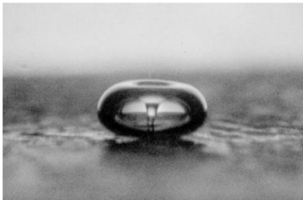
Fig. 30. Jet formation during the collapse of an oscillating gas-vapour bubble at low pressure (4–5 kPa) in a 60 Hz sound field. The bubble size is approximately 0.2 cm (Photograph courtesy of LA Crum). For further details, see the associated web page. 67
