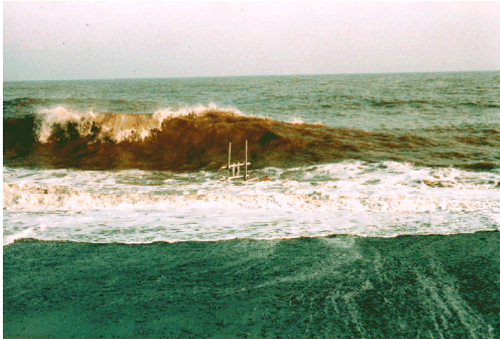
Fig. 9. The first measurement of the bubble size distribution in the surf zone (at Hull, UK, using the technique of Fig. 12(c)). The acoustic detector is the small black circle clamped between the two smaller uprights. The wave measures approximately 10 ft tall. Taken from Leighton et al. 89
