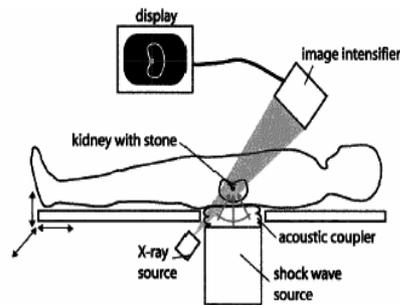
**Figure 1.** Schematic of Lithotripsy.
