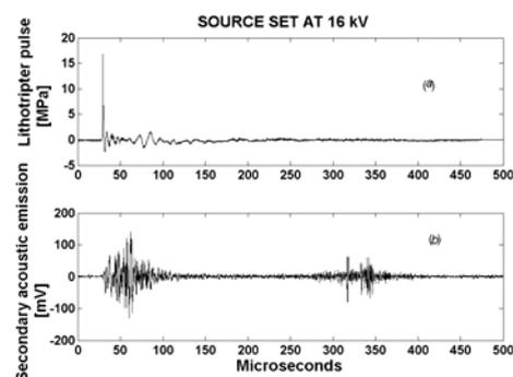
**Figure 4.** (a) Experimental lithotripter pulse at 16 kV. (b) Secondary acoustic emission detected using the NPL cavitation sensor.
