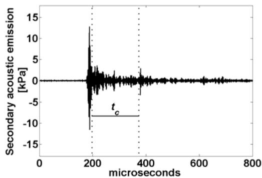
**Figure 6.** Secondary acoustic emission recorded *in vivo* exploiting a PAL calibrated prototype.
