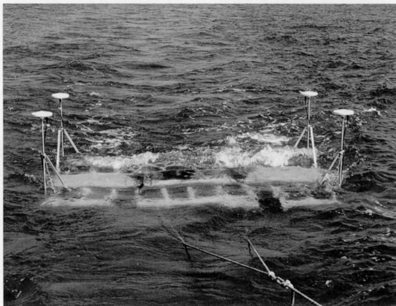
Figure 8. The 3D Chirp array being towed in the Solent, U.K., in August 2003. The four antennas allow the position of the source and each hydrophone group to be accurately known. The array is about 2.7 m across by 2.3 m long.
