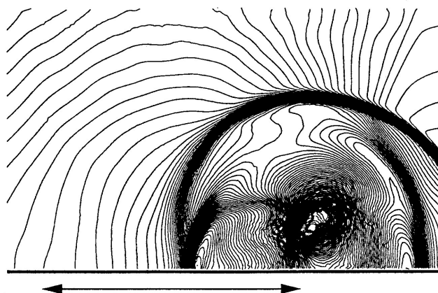
Figure 15. Shock/cavity interaction, t=4.3\mu s . Legend as Fig.2. Air in vortex core at 15000K and 0.4GPa
