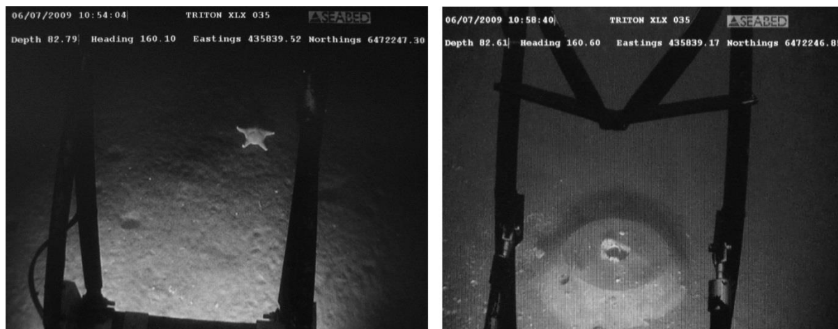
Figure 3.29 Still from the ROV video survey at Sleipner in 2006 showing local fauna (left) and one of the concrete benchmarks from the gravity survey (right). (Images courtesy of CO2ReMoVe project and Statoil ASA).
