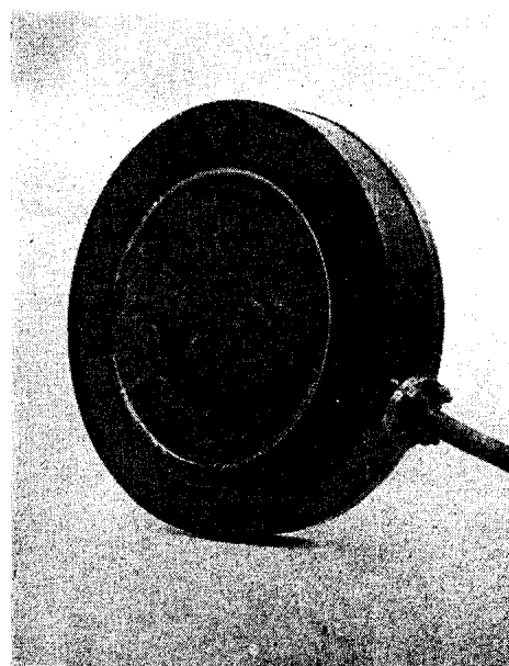
5 inch diameter tourmaline explosion pressure gauge for use with the C.R.O. 1919
