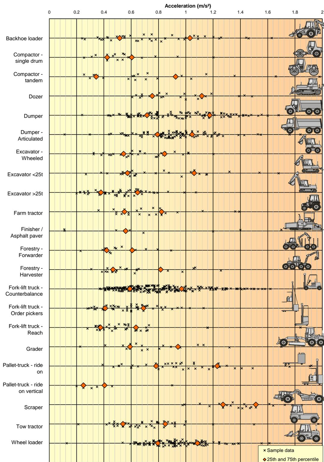
**Figure B.3 Examples of vibration magnitudes for common machines**
