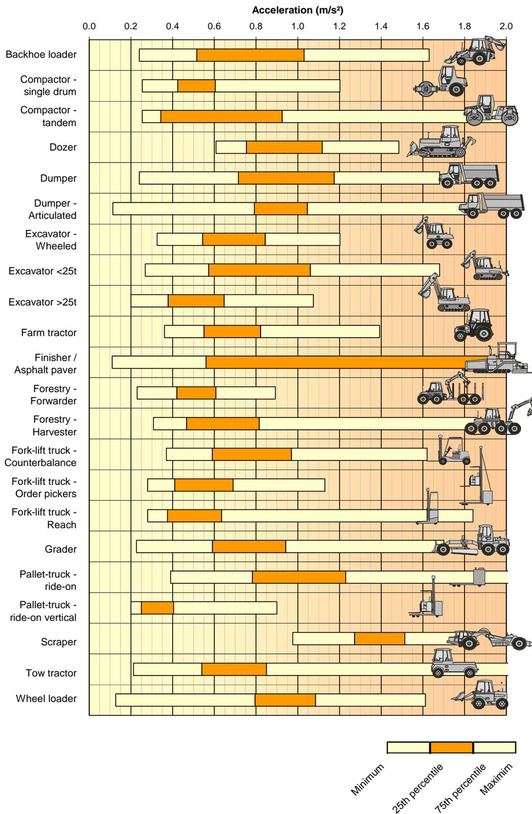
**Figure 2 Examples of vibration magnitudes for common tools**
