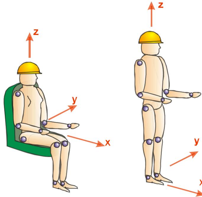
**Figure B.2** Vibration measurement axes
