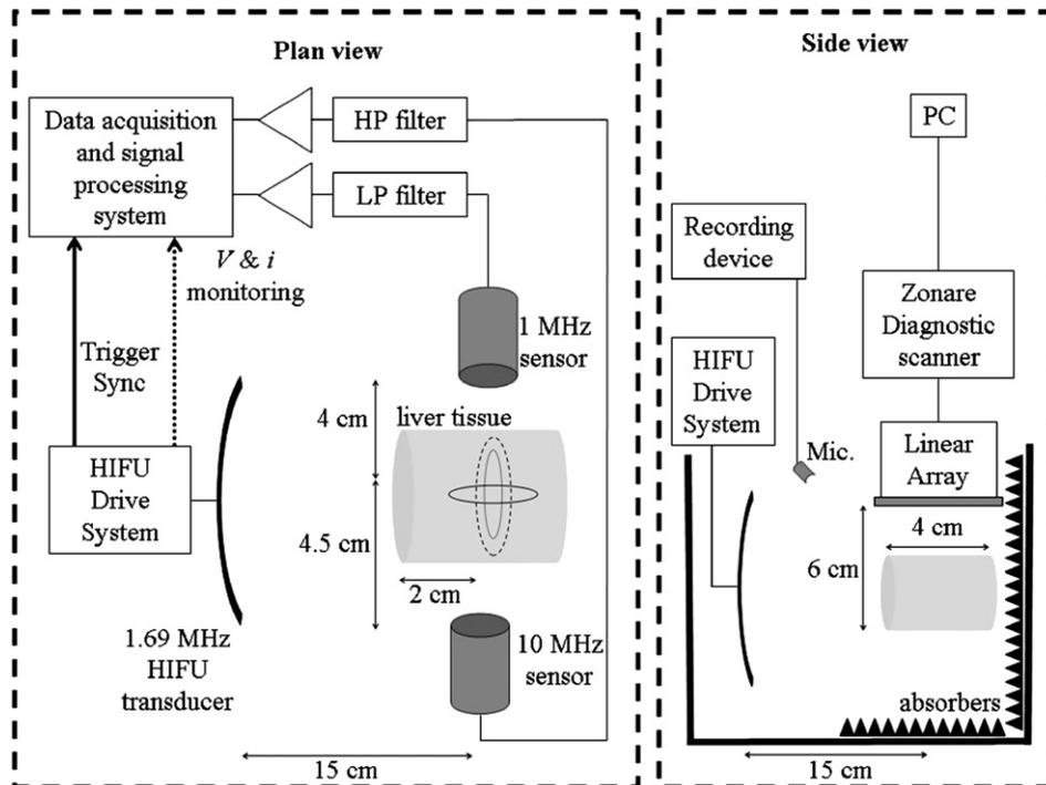
Fig. 1. Plan (left) and side view (right) of the experimental setup used for the degassed water and ex vivo tissue study. The tank is omitted from the plan view for clarity. The relative (to each other) focal sizes of the HIFU (solid line, radial FWHM 2 mm, axial FWHM 16 mm), 1 MHz (dotted line, radial FWHM 4 mm, axial FWHM 30 mm) and 10 MHz (dashed line, radial FWHM 2 mm, axial FWHM 15 mm) transducers are shown.
